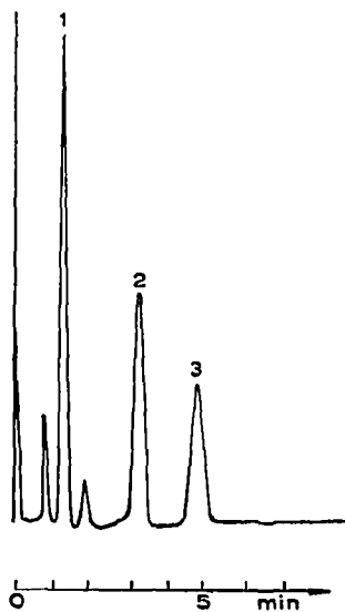
Fig. 3. Separation of HCB from \alpha -BHC by GLC. Column: 2.5% XE-60 on Chromosorb W, 80-100 mesh. For other GLC conditions, see text. Peaks: 1 = HCB; 2 = \alpha -BHC; 3 = \gamma -BHC.
